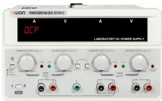
CH1 OCP Protection Alert
